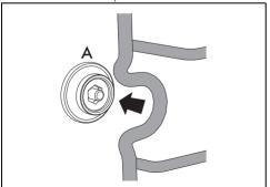
3. Screw in the front fixing pin (you can help yourself with a tool, e.g. a coin).
