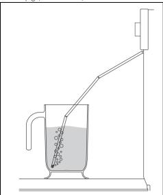
6. Press the start button to start filling the appliance reservoir with water.
