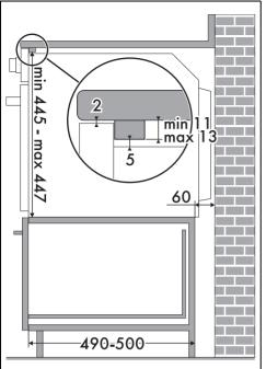
If the appliance is to be built-in under a worktop, a wooden bar has to be installed order to use the seal that is glued to the back of the front panel to prevent water or other liquids leaking in.
