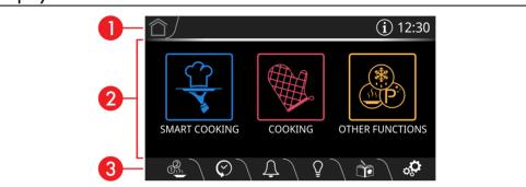
The parameters and values for the currently selected function will be indicated on the display. To use it, simply touch the "virtual" keys and/or scroll through the values indicated (the image shows the main menu screen).
