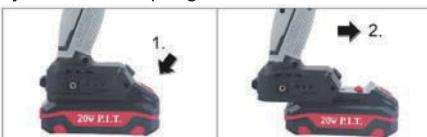
To remove the battery, press the unlocking button and pull out the battery toward the front. **Do not exert any force.**
